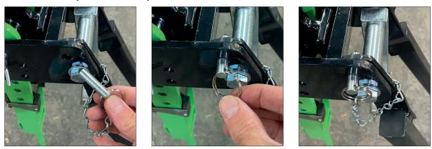
Insert the retaining pin to fix the A Frame in place.
