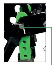
Remove the centre pin to — allow the former disc to be put in place and then replace the centre pin to hold the former disc in position
